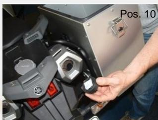
To make sure the second pannier will sit in the same position transfer the holes with a marker onto the back of the second box.
