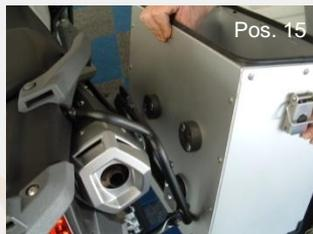
Check if the mountings sit perfect inside the frame of your rack. If not, loosen the screws and move the discs into the proper position.
