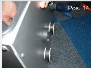
Mount the upper disc with two 6x30mm screws and tighten them until the head sits flat on the black disc. The track head is hit with a hammer into the nylon and secures the bolt.
