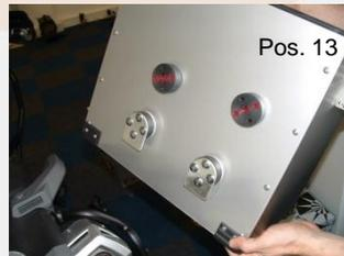
The two holes are drilled into each disc where you marked them and debured from in- and outside.
